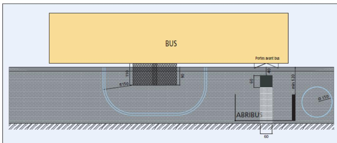
*Figure 10. The layout of tactile surfaces on a bus stop platform in Belgium.*
