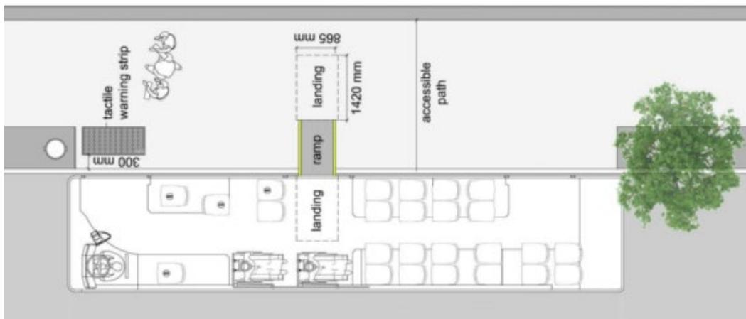
*Figure 15. The layout of tactile surfaces on a bus stop platform in Dubai.*
