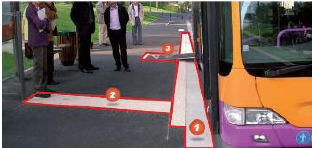
At a bus stop, the blind or visually impaired traveller should be able to identify the position of the vehicle's front door to be close enough to hear the announcement of the line and destination indication (which the fleet of vehicles provides) and be in verbal contact with the driver (CERTU, 2010).
