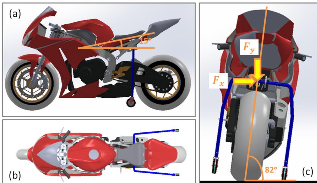
Computer simulations were conducted taken into account Aluminum 6351-T6 alloy and AISI 1060 Steel normalized at  $900^\circ \text{C}$ . The finite element analyses were performed based on the acting stresses and deformations values, with the respective calculation of safety factor for each case. The main mechanical properties (Young's modulus,  $E$ ; Poisson's ratio,  $\nu$ ; and, Yield
