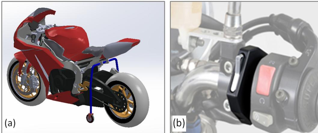
By means of a small electronic circuit, as shown by Figure 4, a 12V DC electric motor starts and keeps activated for a few seconds until the limit switch is activated, being enough for the support to rotate to a partly horizontal position or, in an inverse operation, to a partly vertical position.
