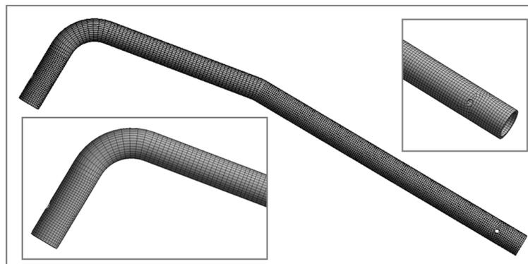
Figure 9. Views of the initial mesh of the caster bracelet.
