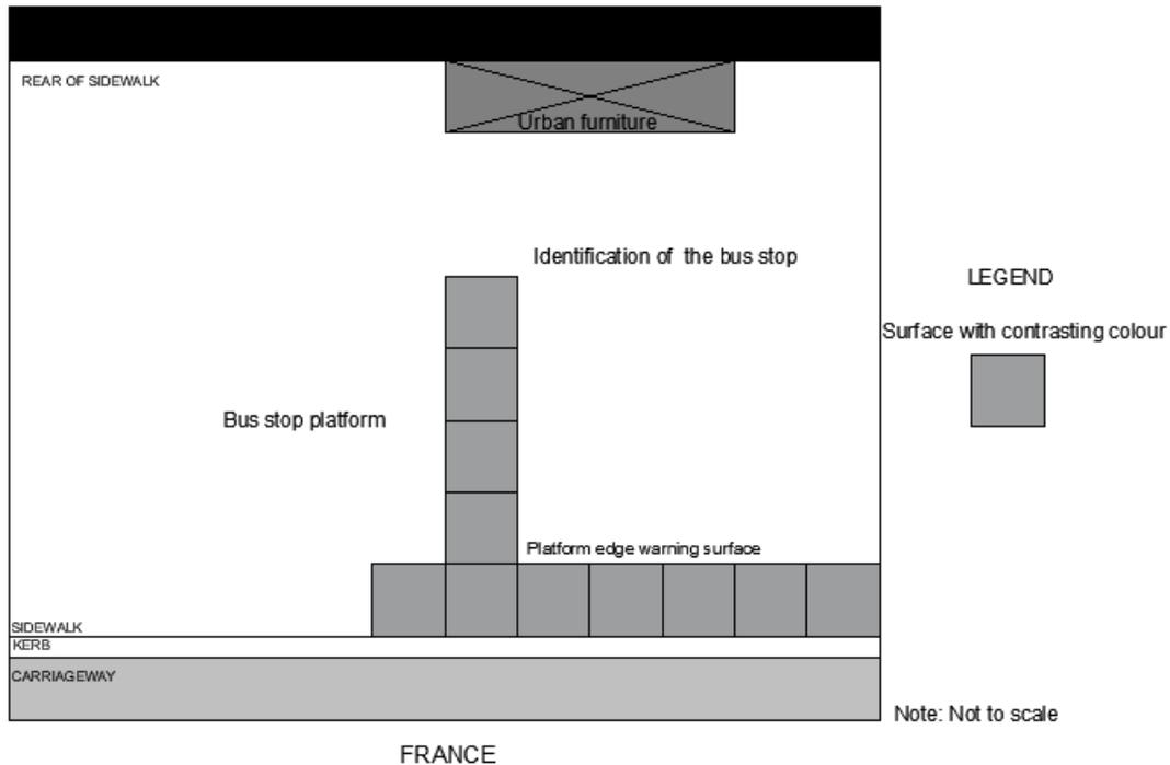
The Norme NF P98-351 frames the use of the tactile bands and considers that the profile of the blister podotactiles comprises rows of rounded blisters with a height of 5mm.
