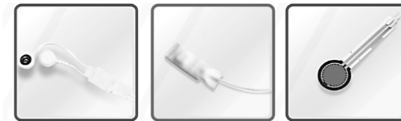
Figure 3. Set of sensors evaluated in our work; from left to right: electromyography sensor, accelerometry sensor, and pressure sensor.
