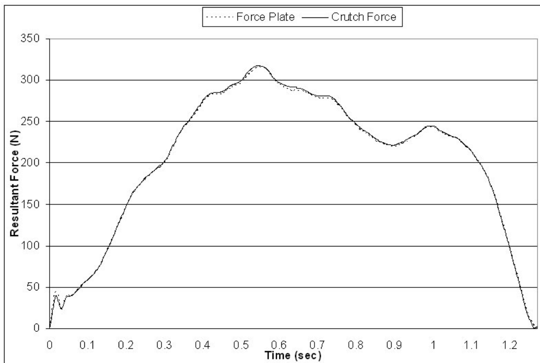
Figure 4. Resultant crutch (solid line) and forceplate (dashed line) forces simultaneously recorded.
